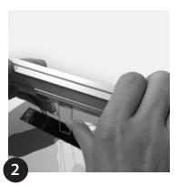
Slide spring clips to ensure even spacing. Compress spring clips, insert into slot and push flush.
